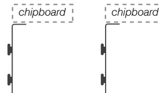
**1.** Attach plastic feet to all 4 uprights, the narrow part of each slot pointing downwards.
